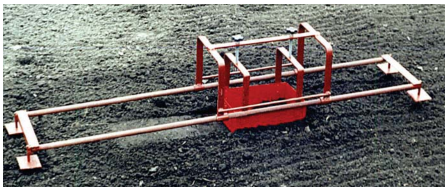
Figure 8 – Device aimed at determination of seed distribution along the furrow depth
